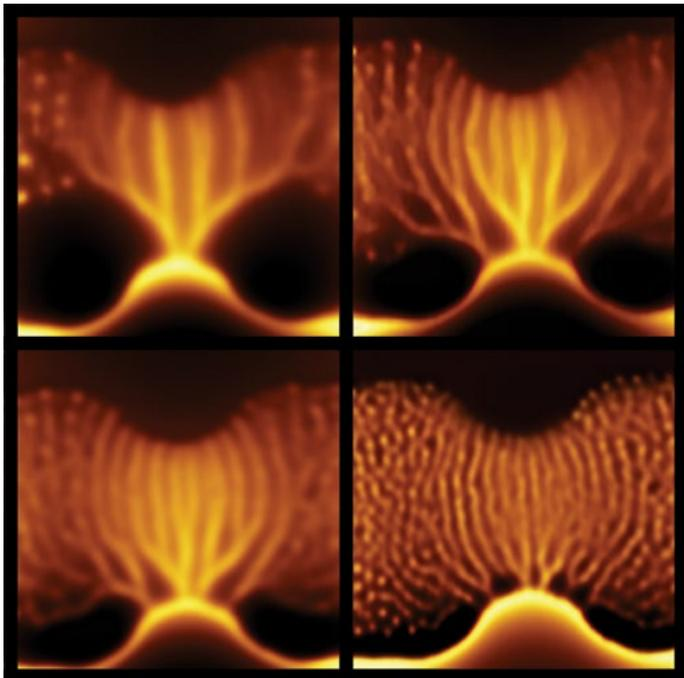
Four different images of vortices penetrating into a superconducting lead film at rates of tens of GHz, and travelling at velocities up to about 20 km/s. The vortex trajectories, appearing as smeared lines, show a tree-like structure with a single stem that undergoes a series of bifurcations into branches. Each image is done at a different magnetic field and each image is 12 x 12  $\mu\text{m}^2$ . (Photo: Yonathan Anahory / Hebrew University)
