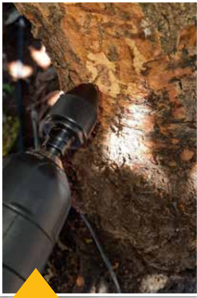
Drilling holes in the stem for the sap flow sensor
