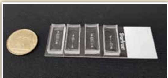
Examples of 3D tumors grown on chip (~300 micrometer)
